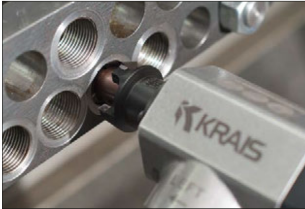
☞ Safely re-machine gasket surfaces in seconds.
