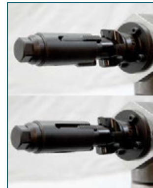
Custom machined jaws. Showing locked and up-locked position.
