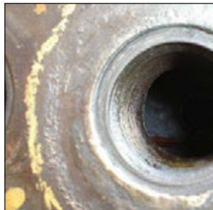
Plug hole before re-machining the gasket seat
