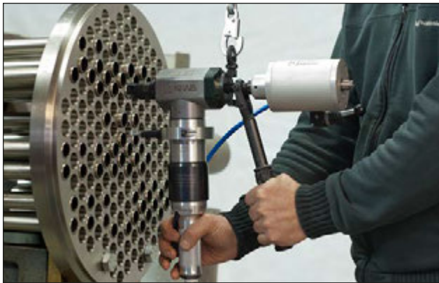
☞ The fast locking and the handle feed make this system very efficient for heat exchanger manufacturers.
